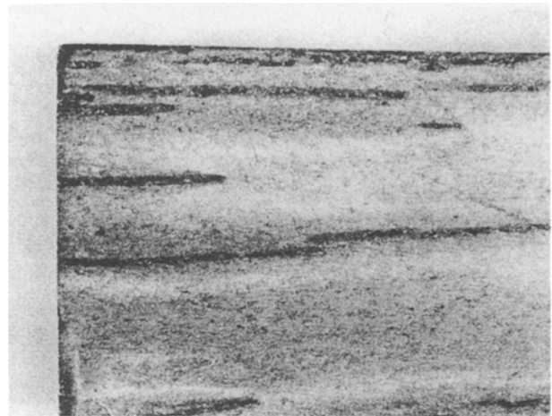
Plate 3 Unreinforced 2014 Al alloy specimen after potentiodynamic sweep ( \times 8 ).
